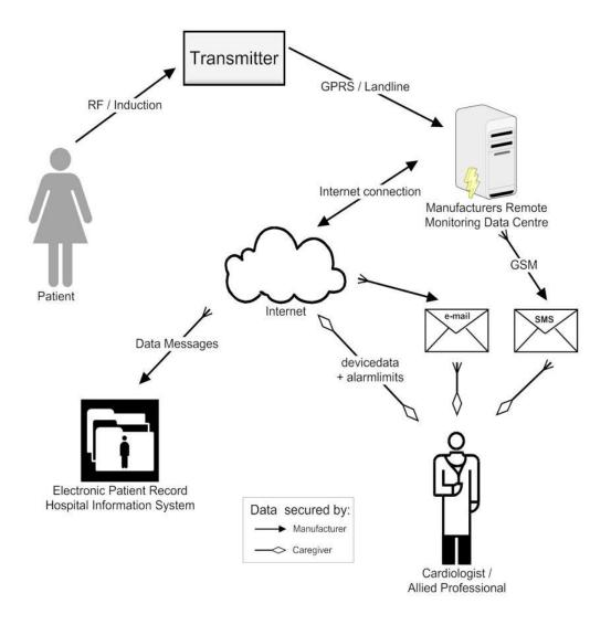
Figure 1. Global overview of remote monitoring and remote follow-up dataflow
